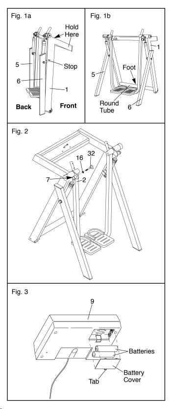
The Electronic Monitor (9) requires two "AA" batteries (not included). Alkaline batteries are recommended. Press the tab on the battery cover and remove the battery cover from the Monitor. Insert two batteries into the Monitor. Make sure that the negative (-) ends of the batteries are touching the springs in the Console. Close the battery cover. and your own phillips screwdriver ()
